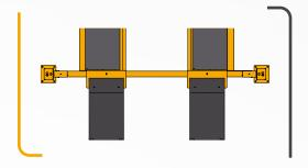
Compatible with pits and scissor lifts, 4-column and parallelogram lift installations. For 4-column lifts, the minimum internal column distance required to operate on production vehicles is of **2900mm.**
